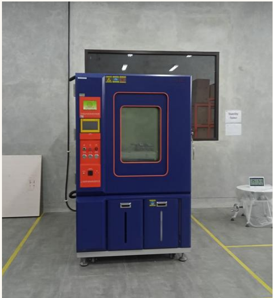
High-Low Temp Humidity Chamber JQTH-1000 Refer to ISTA2A/3A
