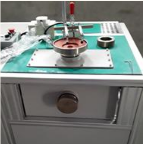
Vacuum Cleaner Test Type Bench Refer to ASTM F558 standards
