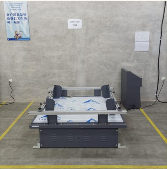
Vibration Tester Machine Refer to ISTA2A/3A
