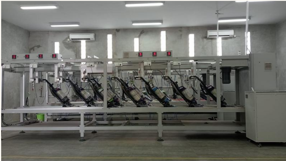
Life Test Machine Capacity 14 pcs / machine Quantity 2 unit machine. TOTAL CAPACITY 28 pcs / Test
