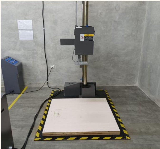
Fall Drop Tester Machine Refer to ISTA2A/3A
