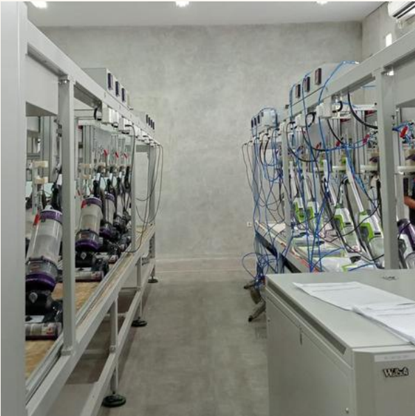
Life Test Machine Capacity 14 pcs / machine Quantity 2 unit machine. TOTAL CAPACITY 28 pcs / Test
